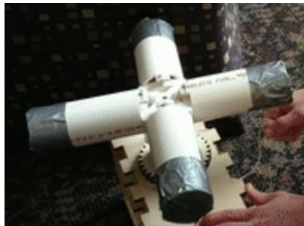
Figure 5b: Assembled flywheel
